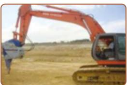
Use of Xcentric ripper in mining operations to reduce noise and vibration
