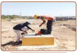
GW monitoring through piezometer
